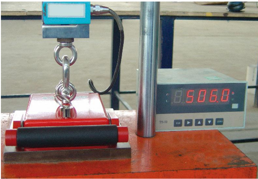
Test-bench verifying magnetic holding force of MAM-003
