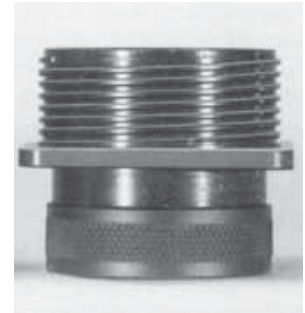
One parallel thread removed to show actual thread angle.
