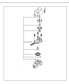
The kit comprises a O-ring for coil, Armature unit assembly, O-ring for the armature unit, spring and diaphragm, two O-rings for the pilot system, and an O-ring and gasket for the equalising orifice.
