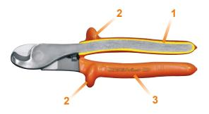
Insulated tools can be identified thanks to the marking on the insulating material. The sign should include a double triangle followed by a 1000V sign and a reference to the standard. In addition, EGA Master tools always include the product reference code and the year of manufacture for a better traceability.
