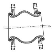
A = Metal Ring B = Flanges = Galvanized carbon steel, drilled acc. DIN-PN 10/16 C = Rubber Bellow Material = EPDM (100°) / NBR (90°) / VITON (200°) \*
