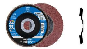
Perfor Flap discs SG A COOL INOX + ALU (Performance Range) Performs exceptionally well on sheet metal and thin sectional material. Specially for stainless steels (INOX), aluminium and non-ferrous metals. Abrasive material: Aluminum Oxide + Coolant. Ensures low build-up of heat in the work pieces when used with minimum contact pressure on variable speed angle grinders at low rpm levels. For weld dressing and surface grinding with low heat input. For aluminium grinding use only grit 40 and 60.
