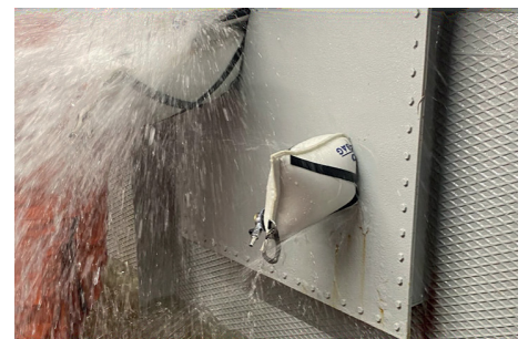
Miko Marine Salvage Bag to control water ingress
