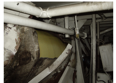
View from inside when the Miko Marine FlexiShape is applied. The Kevlar layer protects against the sharp edges.
