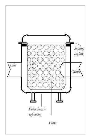
Sea water filters are very varied in appearance, but despite this they contain the same components internally, viz. a filter housing, a filter, an inlet, an outlet, and last but not least, a sealing surface between filter and housing.
