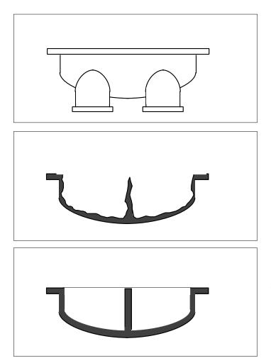
Corroded cooler end covers are very common problems on board a ship. There are several ways of dealing with this. A temporary repair can be made, or the repair can be of a longer lasting nature. The latter method necessitates shot blasting, which as a rule is undertaken ashore. Grinding or needle gunning are other means of carrying out the preparatory work. It is important to remove the graphite as the aim is to obtain a clean metal surface. The inlet and outlet end cover is shown here.
